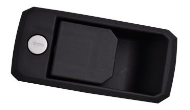
This 030-7150 Plastic Rectangular Paddle Handle is designed for use on personnel and compartment doors for light to medium duty, on or off-road applications. The paddle rotation drives a plunger output which allows for a direct latch release providing a compact and low-cost access solution.
